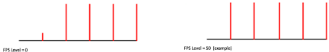
Figure 17: Examples of using the FPS function to control the first pulse suppression.
