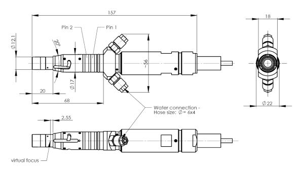
QBH-compatible connector, water cooled
