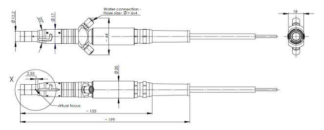
QBH-compatible connector, water cooled
