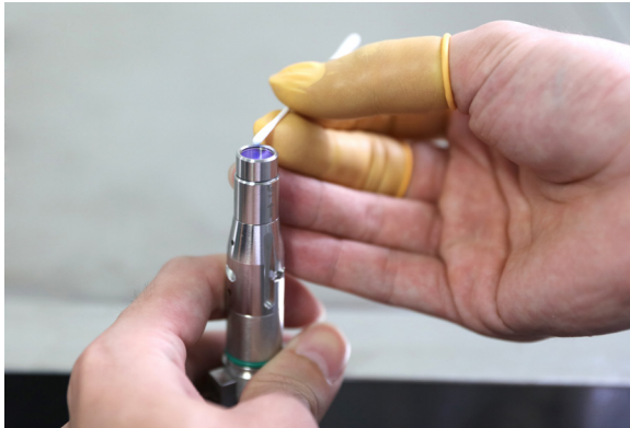
7-3 Cleaning protective lens with swabs
