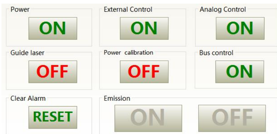
Figure 40 Laser power-on, mode selection, laser emission control display area
